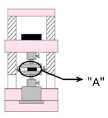
1) Place the test specimen on the perforated suppor -ting plate
